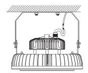
Connect the electrical cables. Brown-L, Blue-N, Yellow/Green-Ground. If using in wet locations, ensure all electrical connections and installation holes have a water tight seal.
