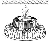
2. Secure hook to the ceiling and hang the fixture from the hook.
