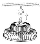
Drill a hole into the ceiling for the appropriate size hook (provided by installer).
