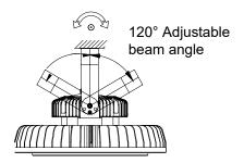
3. Adjust the bracket to the beam angle you need.
