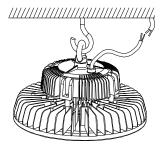
Connect the electrical cables; Brown-L, Blue-N, Yellow/Green-Ground. If using in wet locations, ensure all electrical connections and installation holes have a water tight seal.
