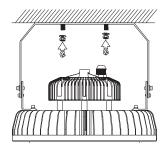
1. Attach the bracket to the mounting surface.
